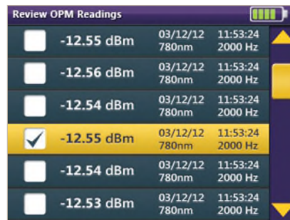
Store Inspection and Measurement Readings on the Device Store up to 10,000 measurement results on the device for export to a PC.
