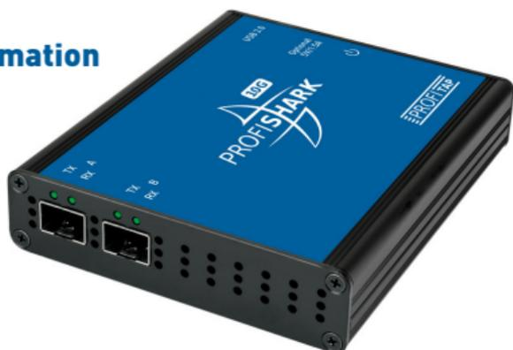
The ProfiShark 10G is a portable fiber optic TAP and troubleshooter, and provides visibility into 10G fiber optic networks. It accepts two SFP+ modules (SR, LR, ER), and sends the incoming traffic to a USB 3.0 output.
