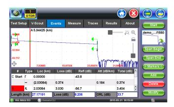
The RXT-4100 OTDR employs specialized techniques developed from decades of experience to locate and measure connectors, splices, optical splitters and macro-bends.
