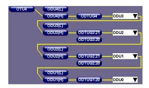
OTU4 multi-step mapping/multiplex structures
