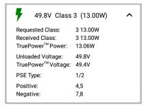
The PoE card displays additional TruePower™ results only if TruePower is enabled in the PoE Settings. TruePower applies a load equivalent to the selected class to mimic a Powered Device (PD).
