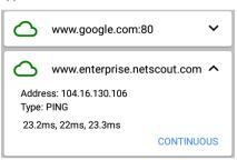
The expanded Target Test card shows the IP address of the target, the type of test (Ping or
