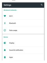
Use the device Settings screen to adjust the LinkRunner G2 display, sound, date/time, and language, view installed applications and memory devices, update your software, or reset to factory defaults.
