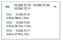
Expand the DNS card to view the response times from each DNS server. The LR G2 pings each DNS server three times and displays the response time from each Ping. Up to four DNS servers are captured and displayed on the DNS test card.
