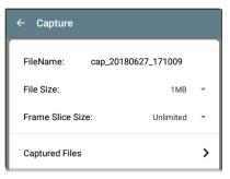
**Filename:** Capture files are automatically named using the date and time. Touch this field to enter a custom name.
