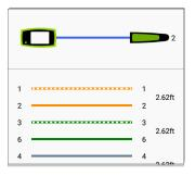
The Wire Mapper Cable Test displays the number of the WireView attached, unless a cable fault prevents LR G2 from detecting the WireView.
