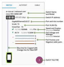
Tap the FAB on the Switch test screen to access the following actions:
