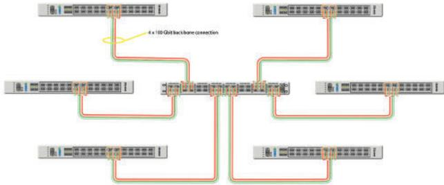
6 x EX20400 are connect over 4 x 100 Gbit to one EX 32100 to build a 500 port 10 Gbit cross connect.
