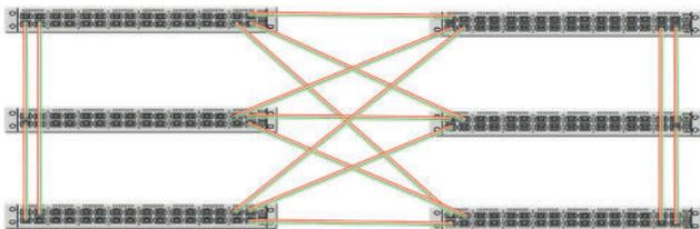
In this application 6 EX 32100 are connected to a fully mached cross connect with 162 available 100 Gbit ports (27 per box).
