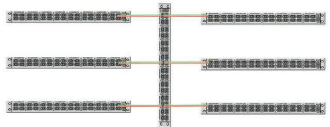
In this application 6 EX 32100 are connected to a central with 186 available 100 Gbit ports (31 per box).
