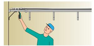
Cable tracing: With TM30 even short underground telecom & mains cables can be traced easily. Below image depicts a typical situation of tracking the route of a street light pole feeding cable with the help of a ground rod.
