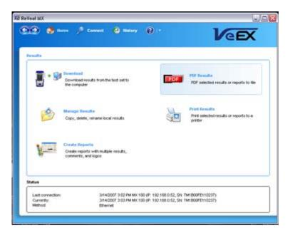
Select PDF Results to generate a PDF file of any results file stored in the PC where ReVeal is installed.
