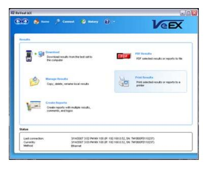
Select Print Results to print available results files stored in the PC where ReVeal is installed.
