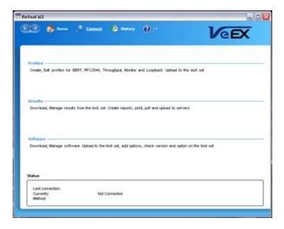
Clicking on Connect will display a Connection Detection window while ReVeal searches for VeEx products (BX100, CX100, CX150, and MX100) on the same subnet/network.
