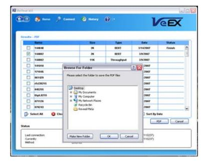
Select the result file to PDF by selecting the check box to the left of the file name. Click on PDF to generate the PDF file and select the location where the PDF will be stored. The default PDF file name is the result file name.
