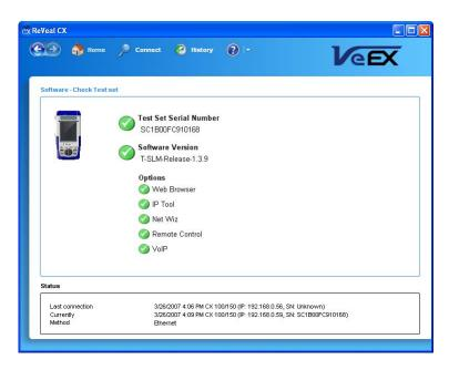
The Check Test Set will display the test set information. The following information is provided: Test Set Serial Number, Software Version, and the Options on the test set.
