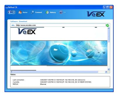
It allows the user to log into the VeEX website to download the latest software version for the test set. Note: the user needs to register in order to access the secure website.
